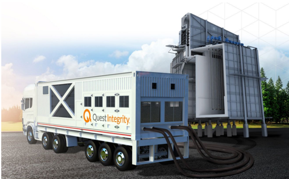
Figure 3. Set Up for Advanced Mechanical Cleaning and FTIS Inspection
