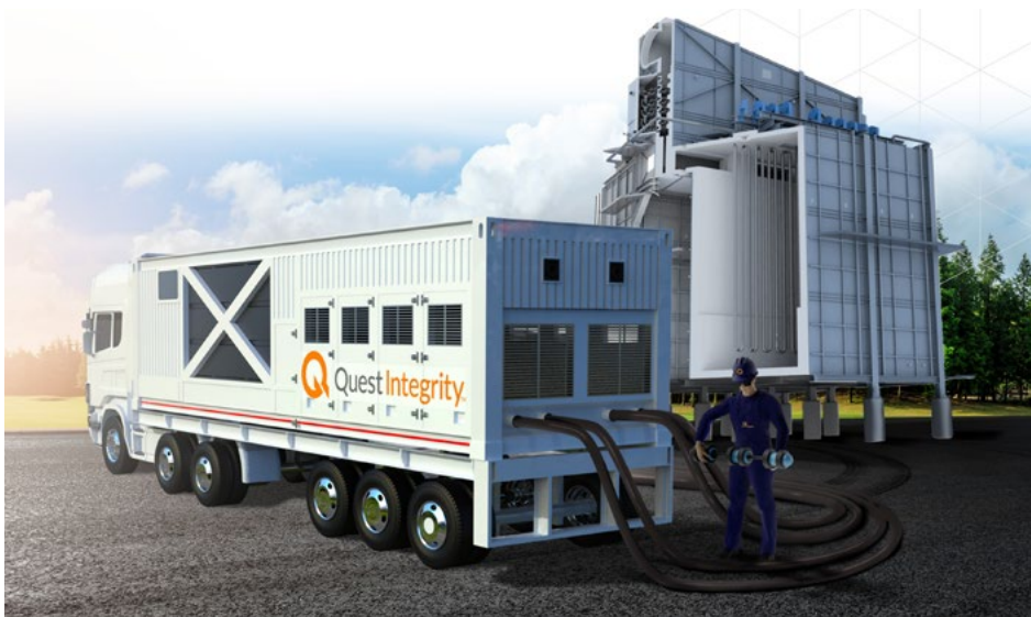
Figure 3. Typical Fired Heater Set Up for Advanced Cleaning and FTIS Inspection
